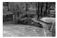
Rain gardens have been especially popular since they can be constructed in various shapes and sizes. Size and placement must fit specific soil types and landscaping. Benefits of a properly installed rain garden include intercepting storm water run-
